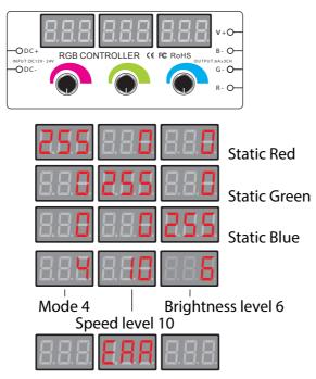
When it is overload or short-circuits, the controller automatically stops output, The indicator blinks "ERR" as above.
